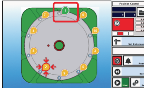
FIRST SCREW COMPLETED (TIGHTENING OK)
